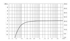
When switch is at 50Hz, it is same as series connecting a 50Hz high pass filter on the input circuit, will attenuate signal under 50Hz, like the pictures
